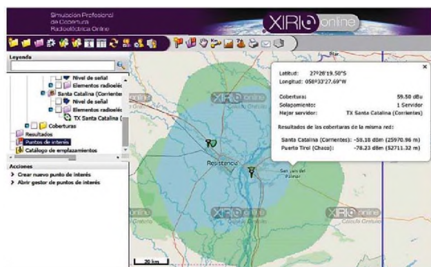
Figura 3: Cobertura multitransmisor red SFN TDA [3]
