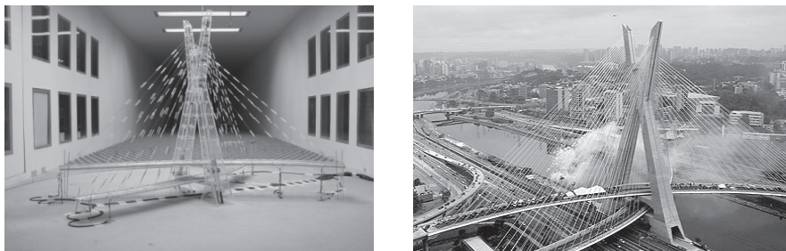
Fig. 4. Cable stayed bridge Octávio Frias de Oliveira, São Paulo, Brazil: (a) full-aerolastic model; (b) real bridge.
