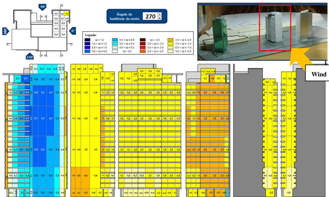
Figure 7. Mean pressure coefficient diagrams on buildings façades from boundary layer wind tunnel tests (suction = red, yellow; pressure = blue) for the central building indicated
