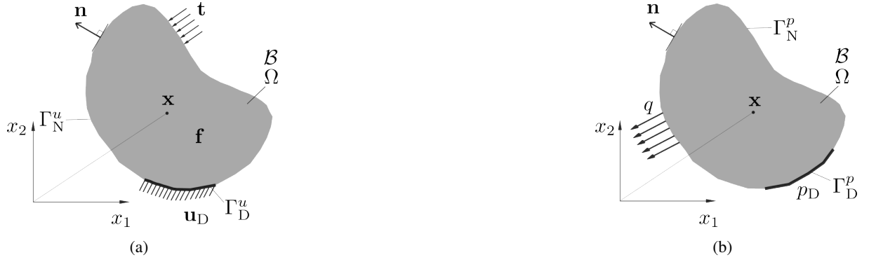
Figura D.1: Macro-scale model layout and nomenclature. (a) Mechanical problem. (b) Seepage phenomenon.
