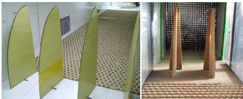
Figure 3. Full-depth Counihan vortex generators in Jacek P. Gorecki wind tunnel (TVG) (left) and part-depth Irwin spires in TV2 wind tunnel (right).
