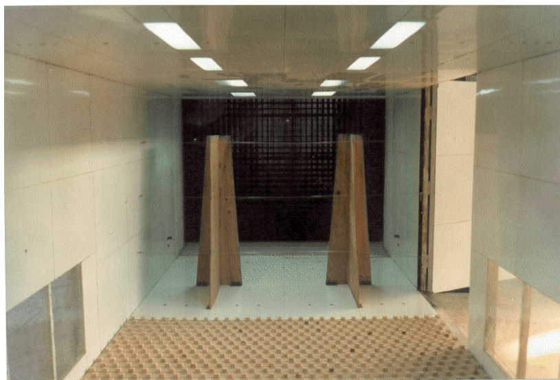
Figure 1. Wind tunnel simulation of the atmospheric boundary layer.
