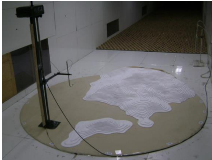
Figure 6. Topographical model inside the wind tunnel (scale 1:2000) [5].
