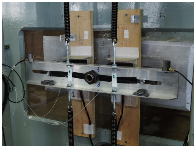
Figure 15. Spring supports of the sectional model [10]
