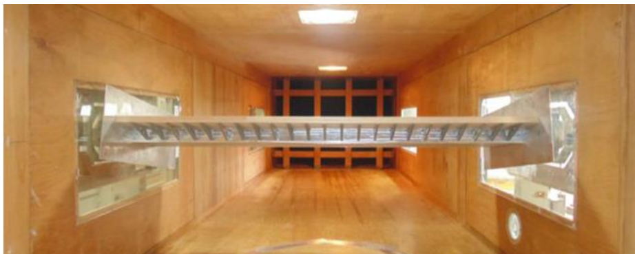
Figure 13. Sectional model inside the wind tunnel [9].
